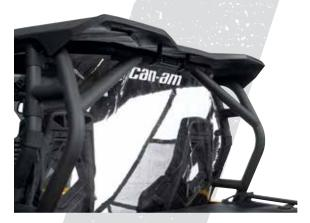
SOFT REAR WINDOW Clear, flexible window made of see-through vinyl. • Resists cold cracking to -4°F (-20°C). · Blocks windshield backdraft or dust and rain from entering, for added cabin comfort. · Installs quick and easily on roll cage. · White Can-Am logo at top, to help maintain clear view.
