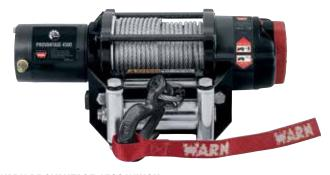
WARN PROVANTAGE 4500 WINCH • Pulling strength capability of 4,500 lb (2,041 kg). • 55 ft. of 7/32" (16.8 m of 5.5 mm) wire steel cable. · Roller fairlead.
